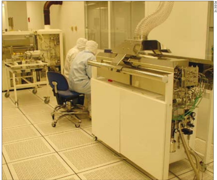
Peide Ye's team at Purdue University is producing inversion-mode InGaAs MOSFETs with minority carrier currents of more than 1 A/mm. These transistors feature gates made from Al 2 O 3 , HfO 2 and HfAlO dielectrics, which are grown by atomic-layer-deposition in an ASM ALD F-120.
